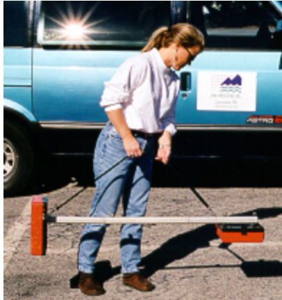
Figure 2.4 - A Deep Focused Metal Detector Being Demonstrated in a Non-environmental Remediation Work Area. (Photo courtesy of Enviroscan, Inc.)
