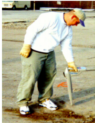
Figure 2.3 - An EM Tracer Being Demonstrated in a Non-environmental Remediation Work Area. (Photo courtesy of Enviroscan, Inc.)
