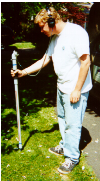
Figure 2.5 - A Vibrocator Being Demonstrated in a Non-environmental Remediation Work Area. (Photo courtesy of Enviroscan, Inc.)
