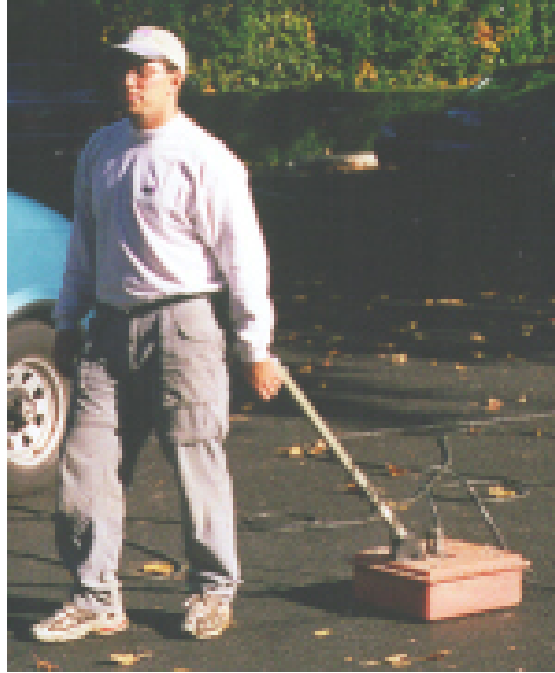
Figure 2.1 - Ground Penetrating Radar Being Demonstrated in a Non- Environmental Remediation Work Area. (Photo courtesy of Envirosan, Inc.)
